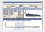
**CSE (Capture Studio Editor)** software enables data captured by Dosimeters and Spectrum Analysers (CESVA SC310, SC-30, SC160, DC112 and VC431 vibrometer) to be edited.
